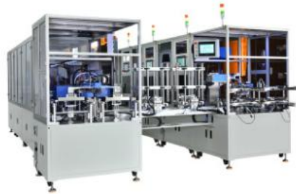
Automatic Laser Soldering Production Line for Winding and Basing of Transformer
