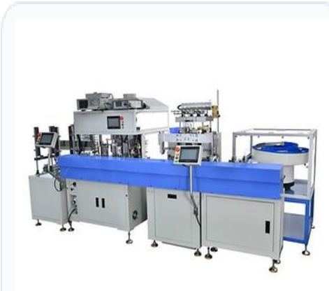
8-spindle automatic valve production line
