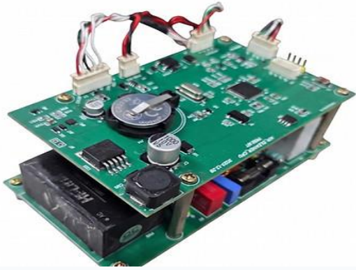
Air Cleaning System -공조기제어시스템
